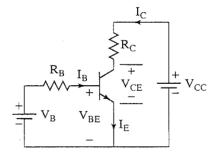
**Q8.** Determine  $I_B$ ,  $I_C$ ,  $I_E$ ,  $V_{BE}$ ,  $V_{CE}$ , and  $V_{CB}$  in the circuit. Assume  $\beta_{DC} = 150$ .
