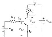
[Ans:  $I_B = 23\mu A$ ,  $I_C = 2.76 \text{ mA}$ ,  $V_{CE} = 3.48 \text{ V}$ ]
