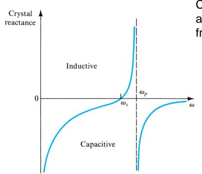
Consists of two resonances such as series and parallel resonance, i.e., two resonant frequencies
