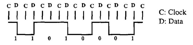
Encoding of the bit sequence "1101 0001" in MFM.
