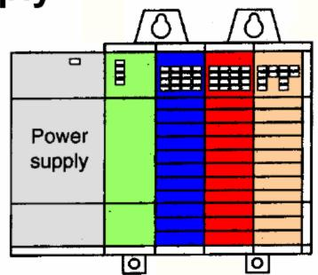
In small and micro PLC systems, the power supply is also used to power field devices.
