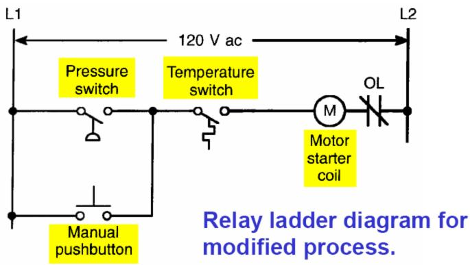
If a relay system were used, it would require some rewiring of the system, as shown, to achieve the desired change.
