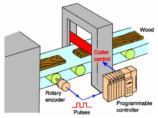
It is easier to create and change a program in a PLC than to wire and rewire a circuit. End-users can modify the program in the field.
