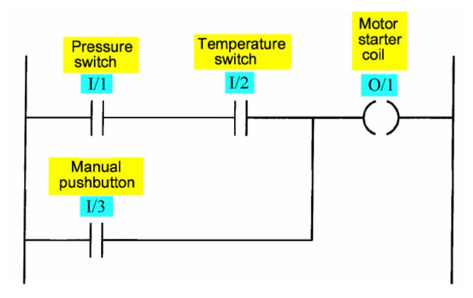
Coil O/1 is energized when contacts I/1 and I/2 are closed or when contact I/3 is closed. Either of these conditions provides a continuous path from left to right across the rung that includes the coil.
