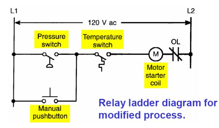
The change requires that the manual pushbutton control should be permitted to operate at any pressure but not unless the specified temperature setting has been reached.
