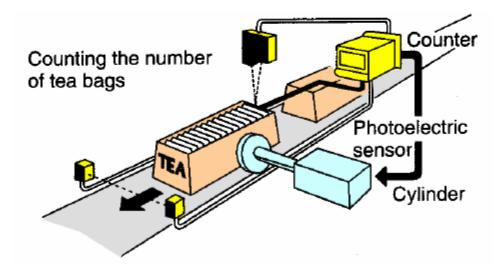
Machines that process thousands of items per second and objects that spend only a fraction of a second in front of a sensor require the PLC's quick response capability.
