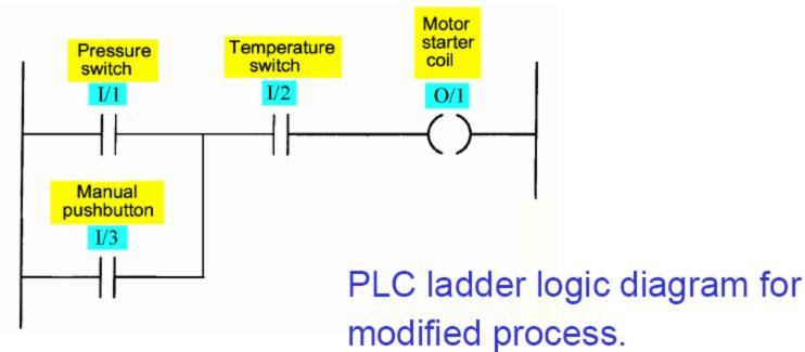
If a PLC is used, no rewiring is necessary! The inputs and outputs are still the same. All that is required is to change the PLC program
