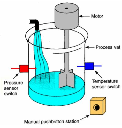
The temperature and pressure sensor switches Manual pushbutton station close their respective contacts when conditions reach their preset values
