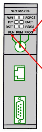
To enter the program into the PLC, place the processor in the PROGRAM mode and enter the instructions one-by-one using the programming device
