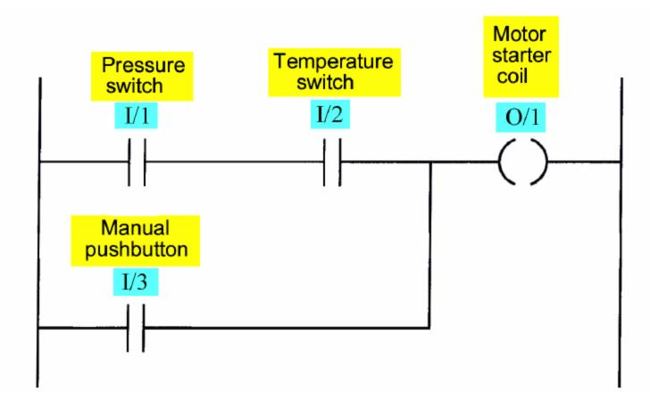
The format used is similar to that of the hard-wired relay circuit
