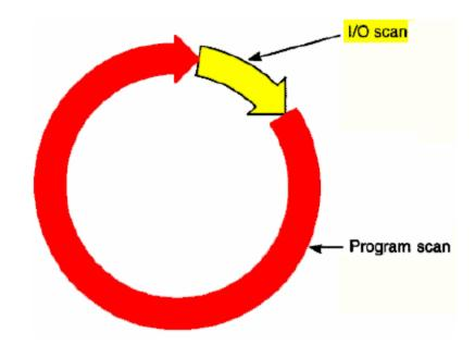
The completion of one cycle of this sequence is called a *scan*. The scan time, the time required for one full cycle, provides a measure of the speed of response of the PLC
